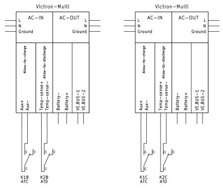
Overview of the relay contacts connected to the Multis.
