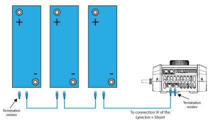
Do not forget the termination resistors at the ends of the CAN-Bus network.
